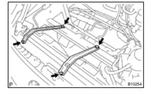
(b) Install the 2 spear wheel carrier extensions with the 2 bolts and 2 nuts.
